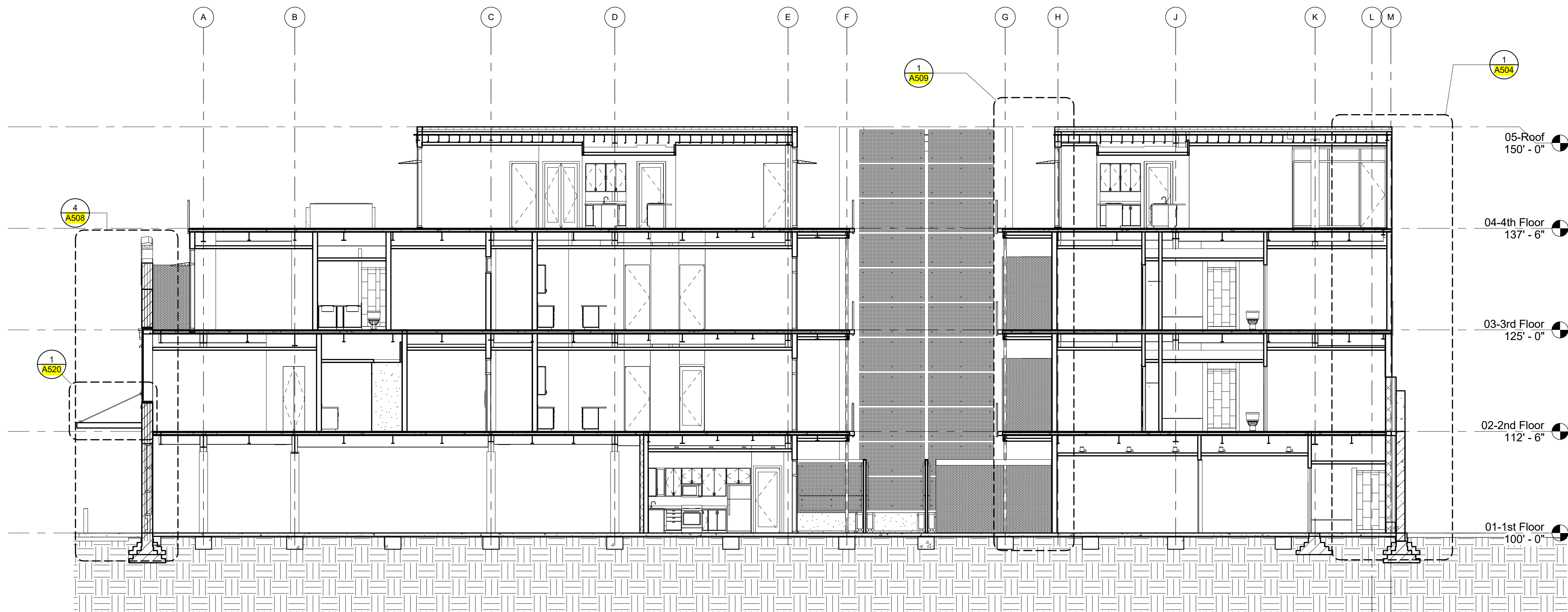
2 LATERAL BUILDING SECTION AT COURTYARD SCALE: 1/8" = 1'-0"
